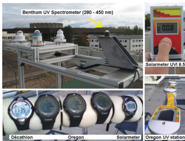
Fig. 1 Instruments used in the intercomparison experiment. (a) Bentham spectrometer, (b) watches with UV sensors of different brands, (c) weather stations with UV sensors, (d) handheld UV sensor.
