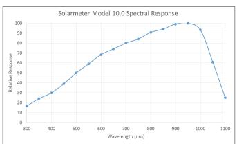
Fig. 1. Model 10.0 Spectral Response
